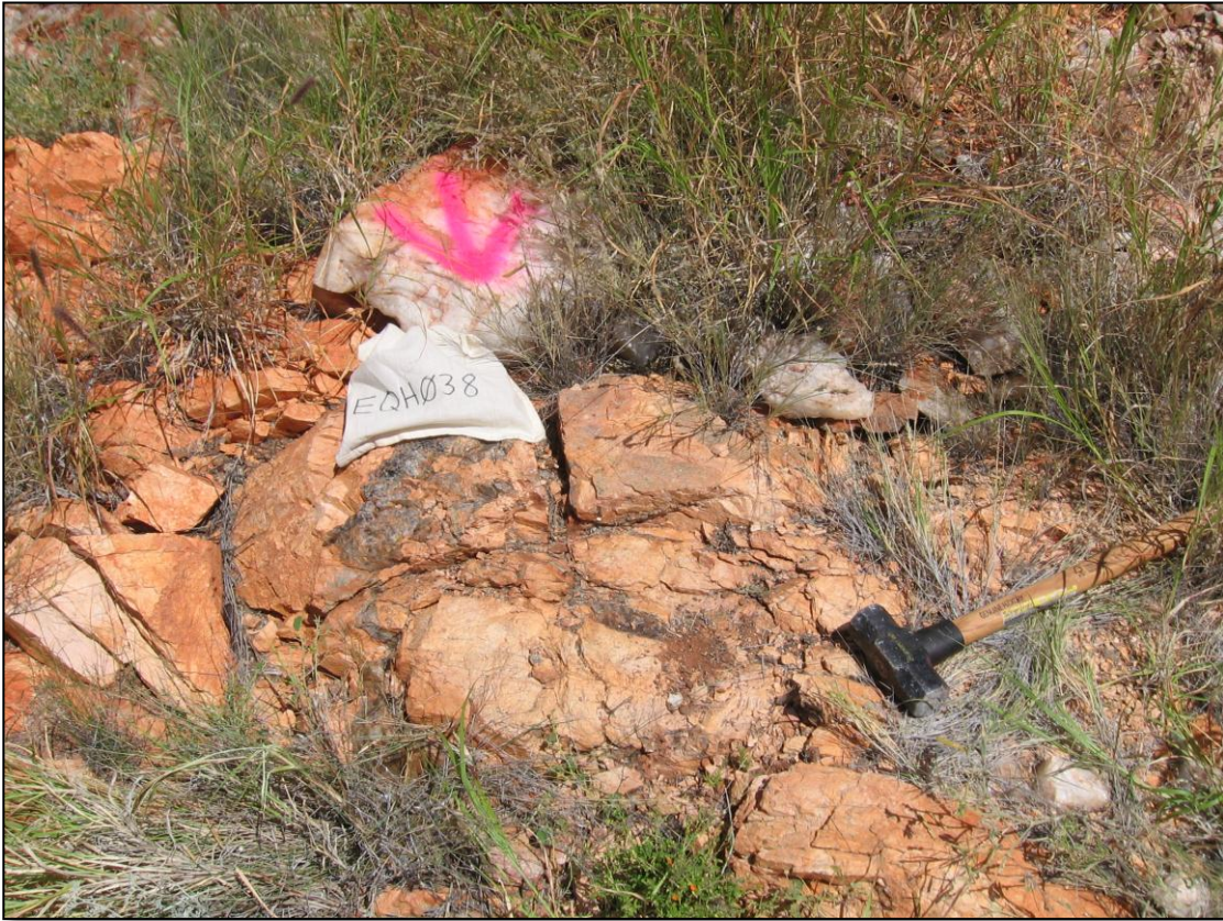
Figure 3: Sample EQH038 – Quartz Hill: This sample was taken from a previously record samarskite occurrence on the north flank of a quartz-rich pegmatite which forms Quartz Hill.
