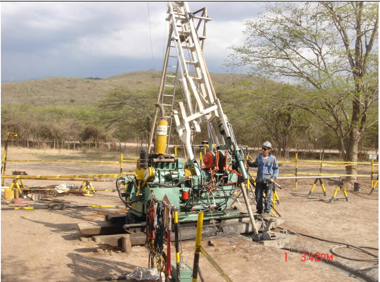
Figure 3: One of two Longyear-38 drill rigs to be used at El Balsal
